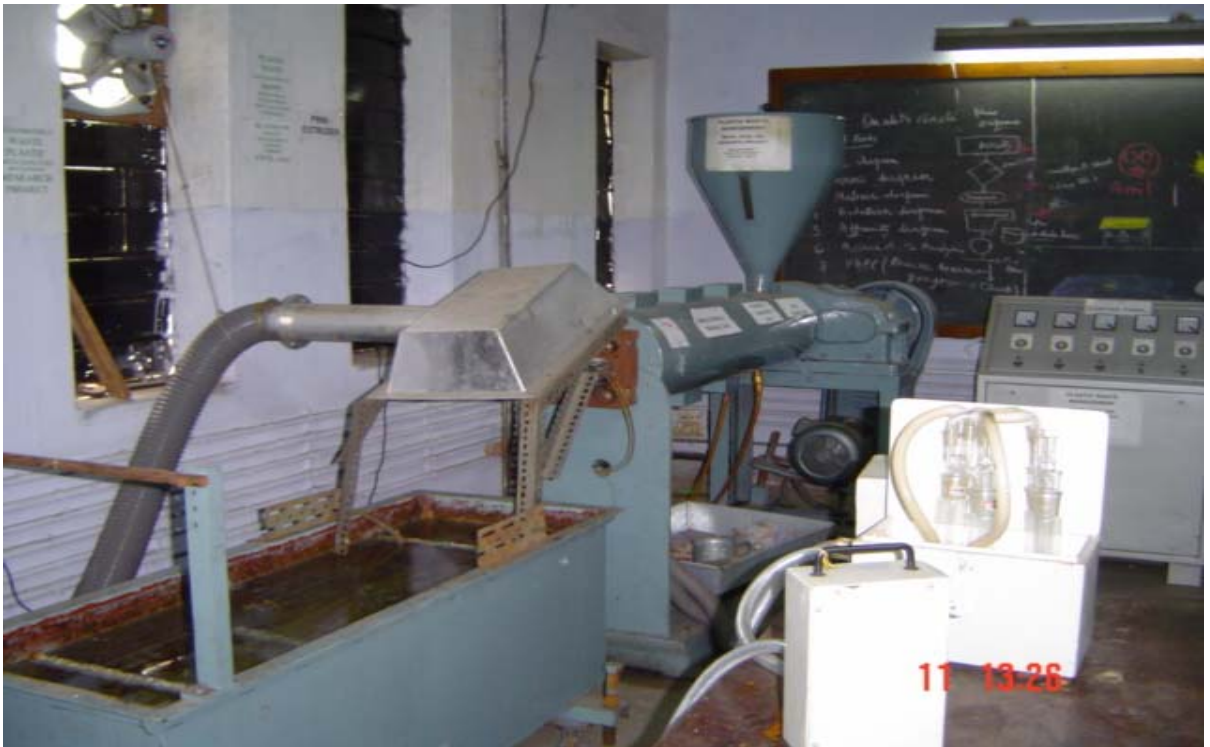
Photo: The Newly Developed Pilot Plant (extruder, control panel & part of pollution monitoring System.
