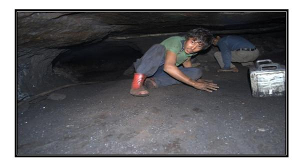
In **box-cutting method** the land is, first cleared by cutting and removing the ground vegetation and then pits ranging from 5 to 100 m<sup>2</sup> are dug vertically into the ground to reach the coal seam. The depth of the vertical shaft varies from 20 m to 130 m depending on the depth of the coal seam. Thereafter, horizontal narrow tunnels are made into the seam. The height of the tunnel, in most cases is about 3 to 4 feet due to thin coal seems.
