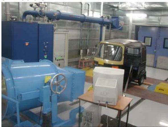
**Figure 18: Schematic of 3-Wheeler Test Cell**
