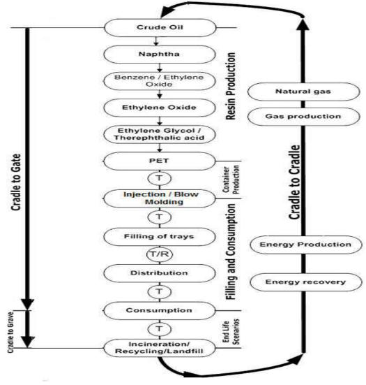
Figure 5: Flow diagram of LCA of PET bottles.
