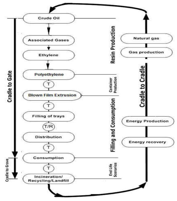
Figure 6: Flow diagram of LCA of milk pouch.
