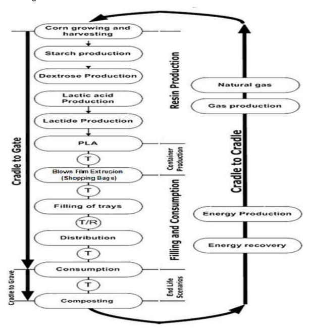
Figure 12: Production of PLA – non-solvent process
