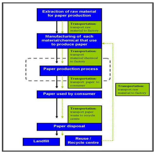
Figure 9: Flow chart for LCA of paper bag process
