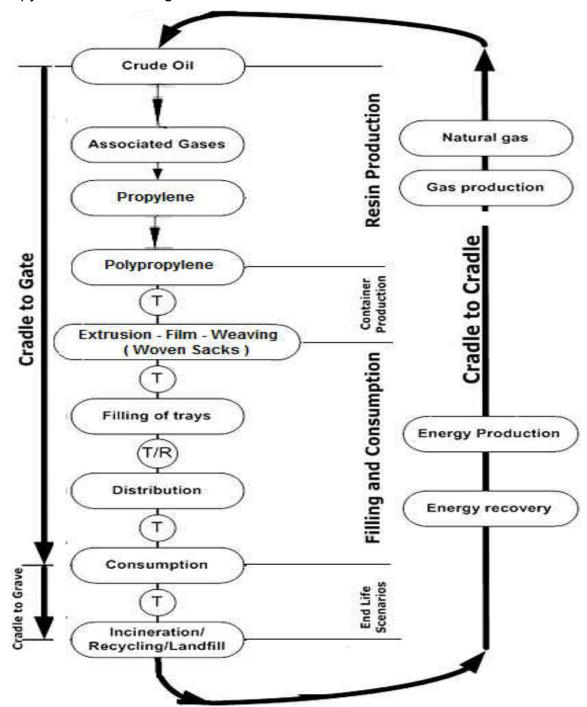
Figure 8: Flow chart of manufacturing process of PP woven sacks.
