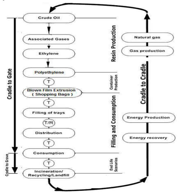
Figure 10: Flow chart for LCA of HDPE bag process
