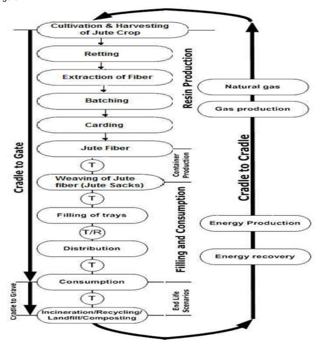
Figure 7: Flow chart of manufacturing process of jute bags.
