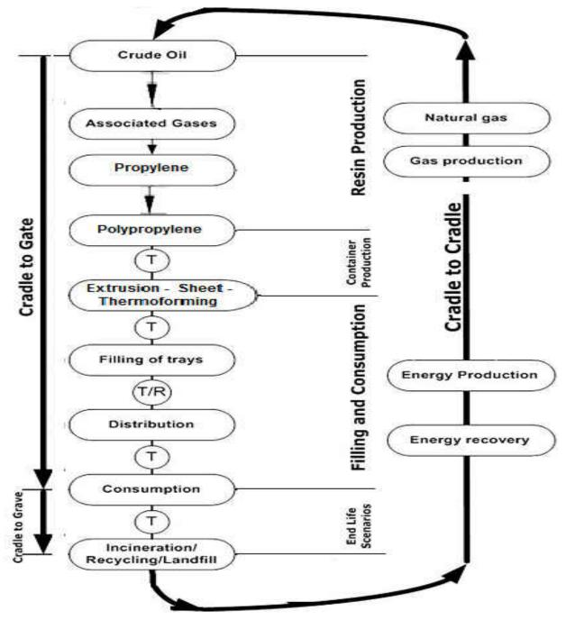
Figure 11: Flow chart for LCA of PP cups.
